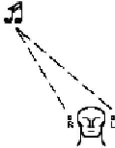
Figure 3: The distance from the sound to R is shorter than the distance to L. Hence, the sound will be played at a louder volume in the right channel, giving the illusion the sound is to the right.
